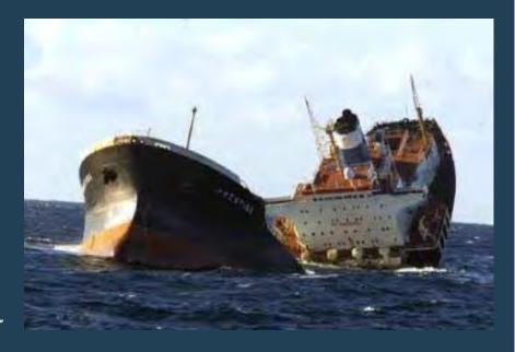
The break-up and sinking released about 63.000 tonnes of cargo. Over the following weeks oil continued to leak from the wreck.
